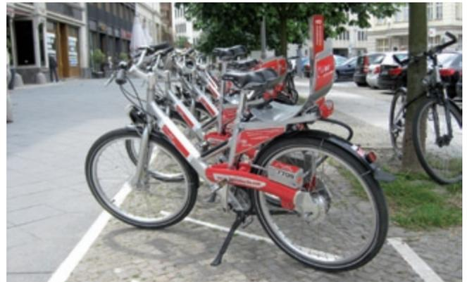
Figure 69: Station without Physical Docking Points (Photo: DB Rent)
